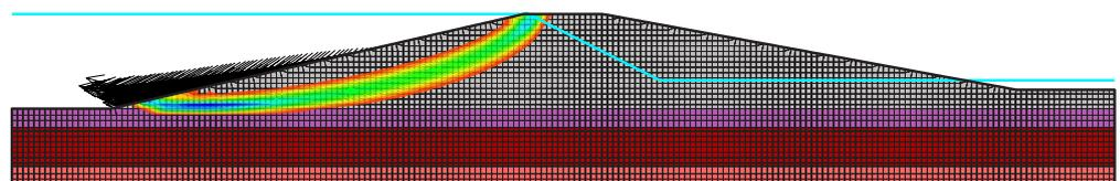
▲ FLAC/Slope model of a dam showing the model view (top); water table, pore pressures, and applied forces to represent the water head above the dam (middle); and the resulting maximum shear strain rates and velocity vectors (bottom). The calculated FoS is 2.45 for this model.
