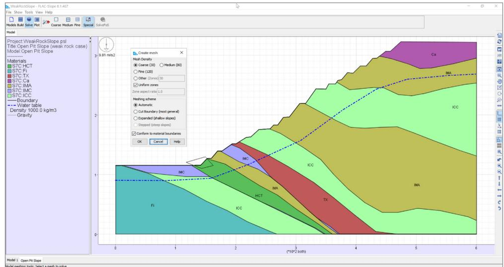
▲ FLAC/Slope user interface showing the model pane with the Create mesh dialog open. Geotechnical unit materials, the water table, and an excluded region (the polygon near the slope toe) can also be seen.
