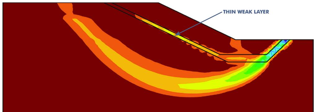
▲ *FLAC/Slope* model of a slope with a thin weak layer. Where the ratio of cohesive strength is 0.6 between the thin weak layer and the surrounding clay, a FoS of 1.37 is predicted. Additional modeling where the ratio of cohesive strength between the weak layer and the surrounding clay of 1.0 and 0.2 results in different failure mechanisms and a calculated FoS of 1.45 and 0.54, respectively. In the latter case failure was confined within the thin weak layer only.
