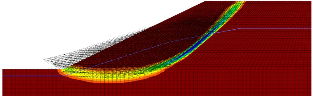
▲ *FLAC/slope* models of a simple slope consisting of two soil types without (top) and with a water table (below). The predicted FoS without and with pore pressures are 1.62 and 1.45, respectively. The presence of water drives possible slope failure mechanisms much deeper through the lower soil towards the slope toe.
