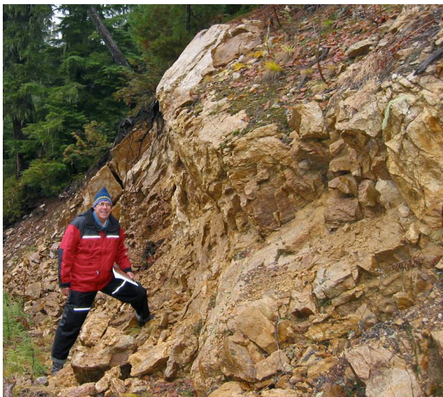
Slope weathered rocks and prominent jointing.
